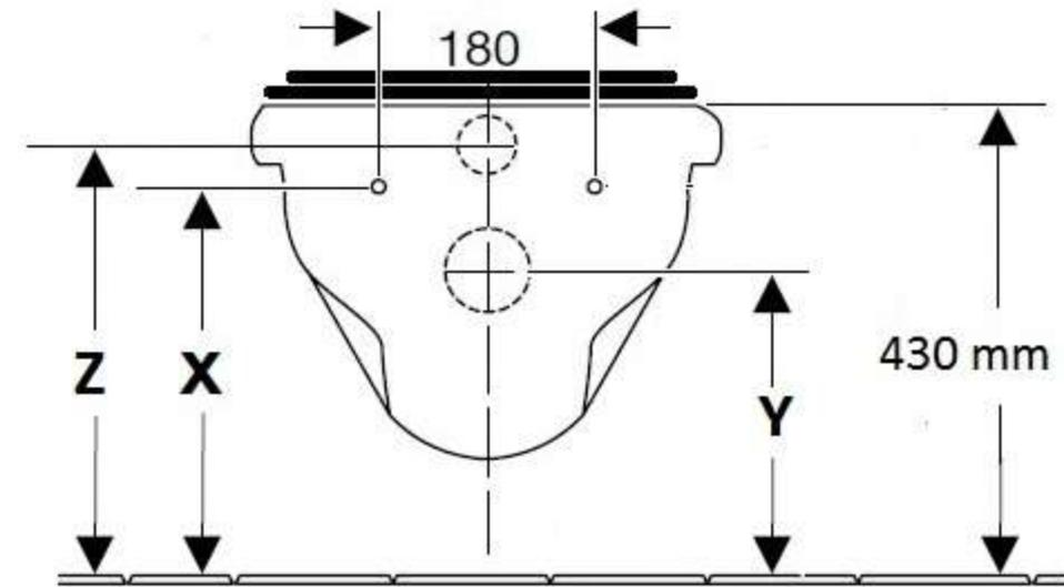
**Fix the rag-bolts in the wall at the distances as per the dimensions of the products. Follow the same procedures for the inlet and outlet holes.**
