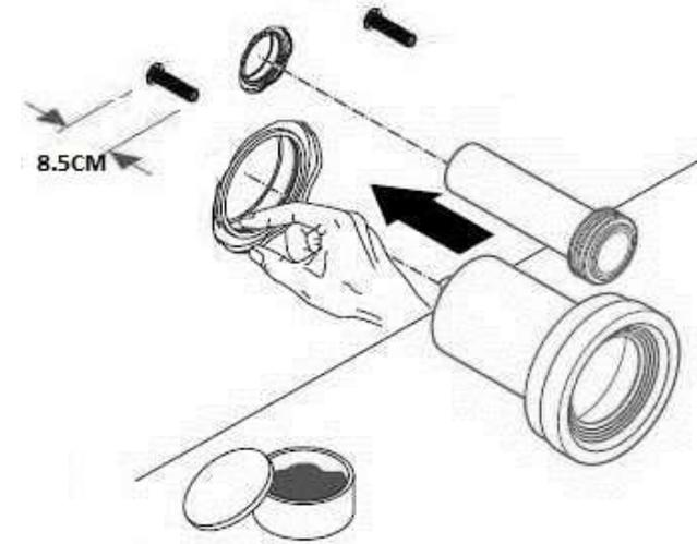
**Ensure that the rag-bolts are projecting to a distance of at least 8.5 cm from the walls. After fixing the connectors, fix the closet in the rag-bolts.**
